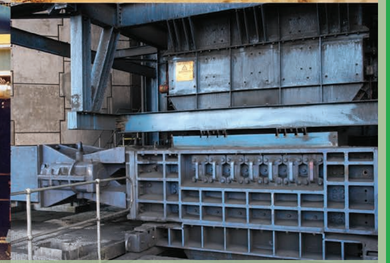
Coal | South Africa | In: 1,000mm | Out: -250mm | Capacity: 2,000TPH
