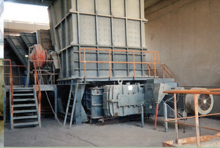
Limestone | Lebanon | In: 800mm | Out: -300mm | Capacity: 1,500TPH
