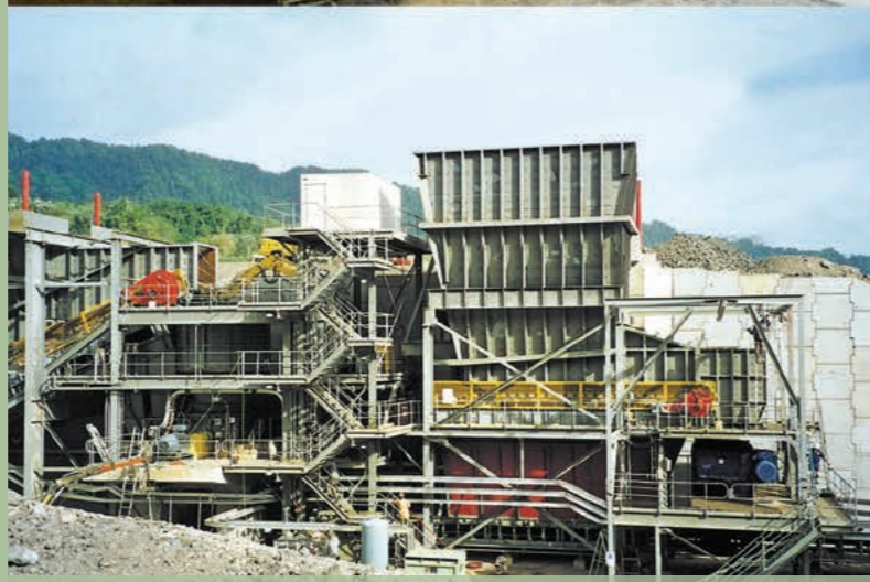
Clay/Gold Ore | Papua New Guinea | In: 600mm | Out: -250mm | Capacity: 600TPH
