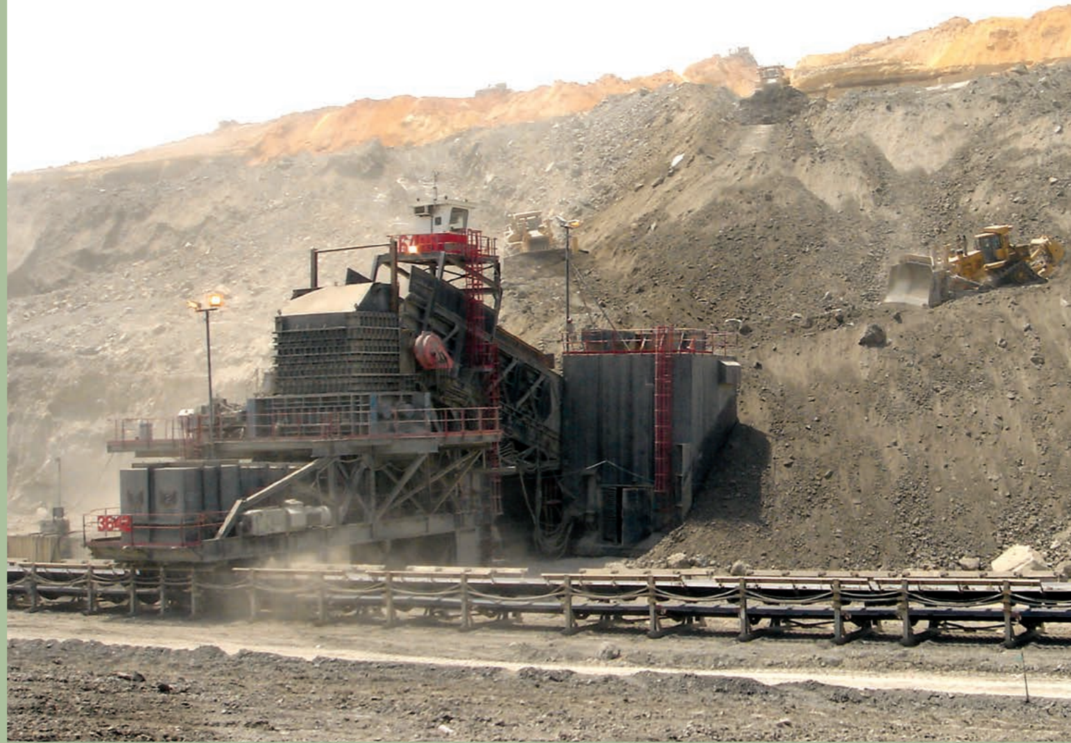
Overburden | Colombia | In: ROM | Out: -450mm | Capacity: 20,000TPH
