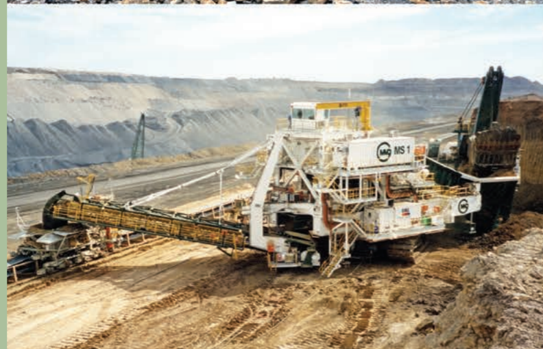
MS1 Fully Mobile Slewing Station | 1400 Series Sizer | D9 Apron Plate Feeder
