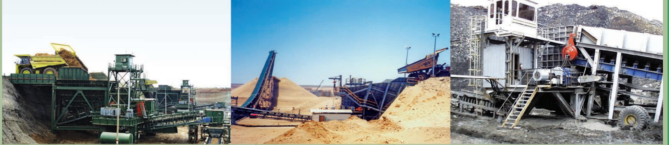
Overburden | Thailand | In: 1,200mm | Out: -400mm | Capacity: 6,500TPH
