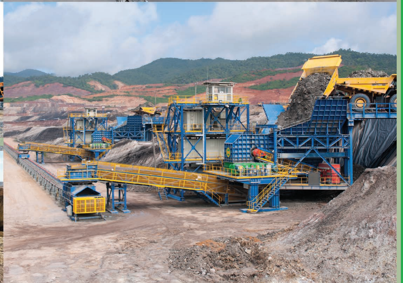
Semi-Mobile Sizer Station with twin truck bridges | 1150 Series Sizer | D7 Apron Plate Feeder
