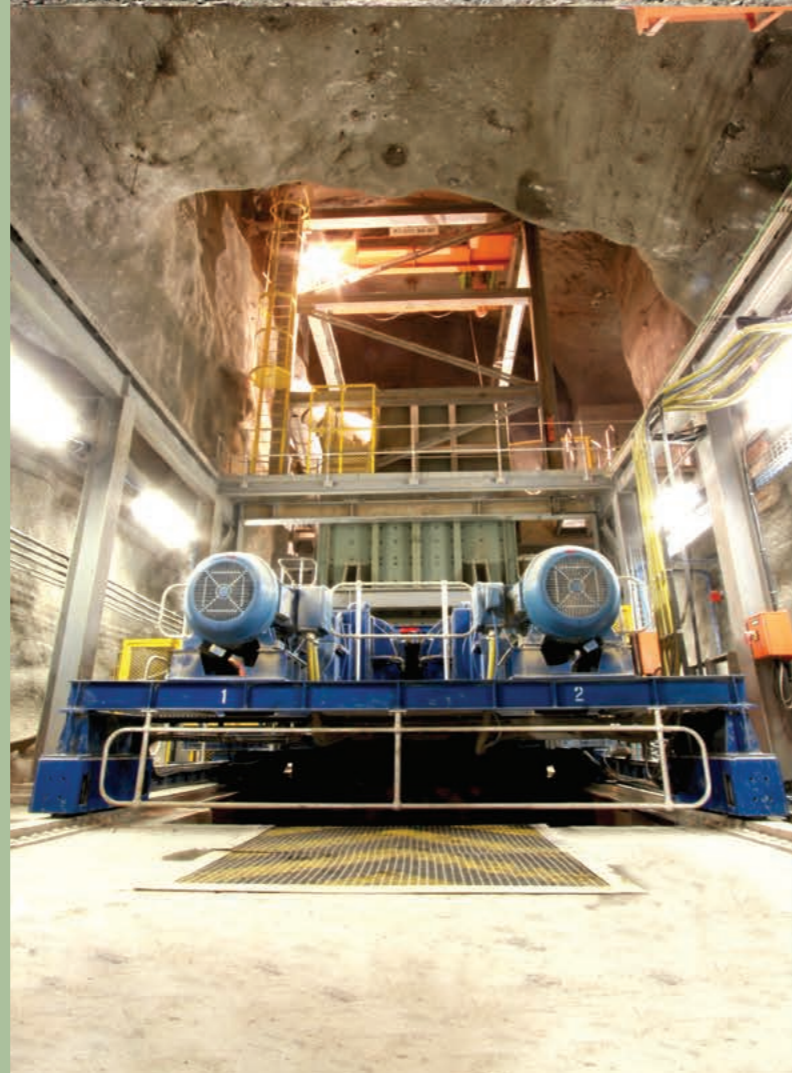
Kimberlite | South Africa | In: 2,000mm | Out: -300mm | Capacity: 800TPH
